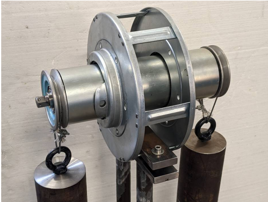
Photo N°10 – Spring box 280x101 with Masinara Nylon rollers
