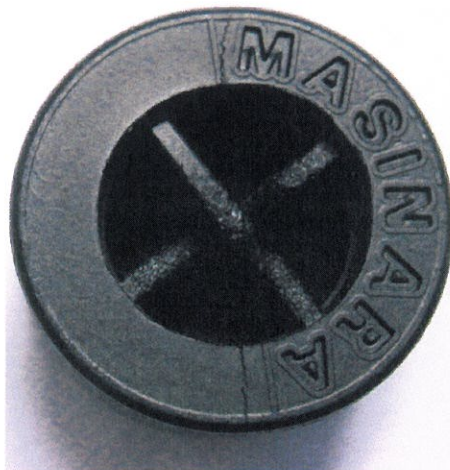
Picture N° 6 After -30° C: breaking begins at 256 daN (=251.14Kg)
