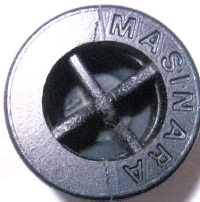
Picture N° 4 T. 25°C: breaking begins at 266 daN (=260.95Kg)
