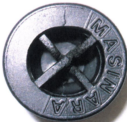
Picture N° 4 T. 25°C: breaking begins at 266 daN (=260.95Kg)
